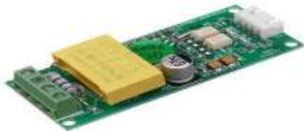
Fig 10: PZEM-004T single-phase AC energy meter sensor module with integrated current transformer and UART interface.
