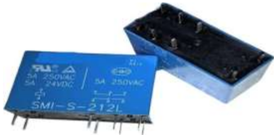
Fig 6: Double Pole contact electromechanical relay module (SMI-S-212L) rated 5 A at 250 V AC .
