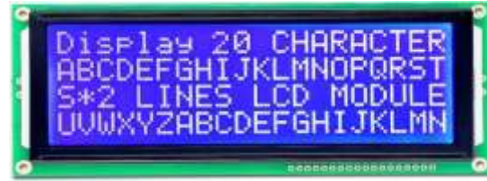
Fig 11: 20" \times 4 character I2C LCD module used for onsite display of electrical parameters.
