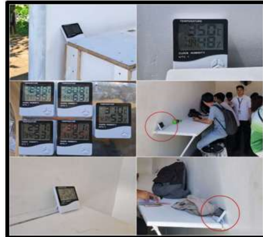
Fig. 4. Temperature data gathering inside the mobile study shelter.
