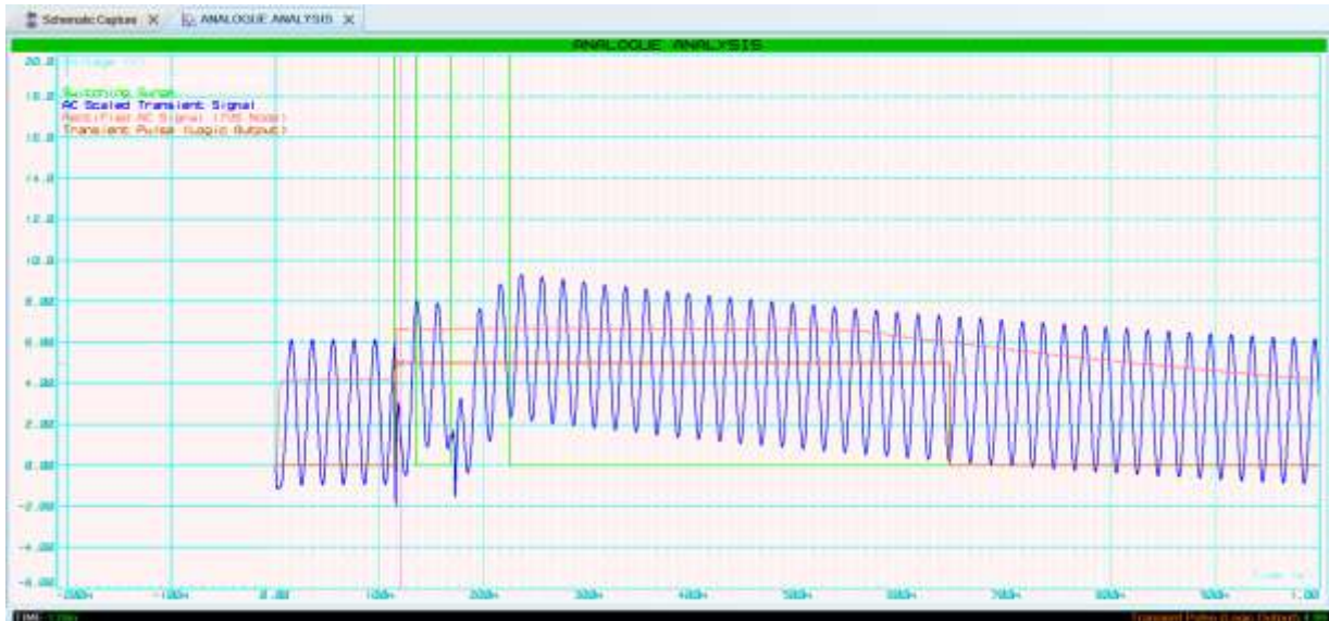
Figure 8: Signal waveforms at transient overvoltage event.
