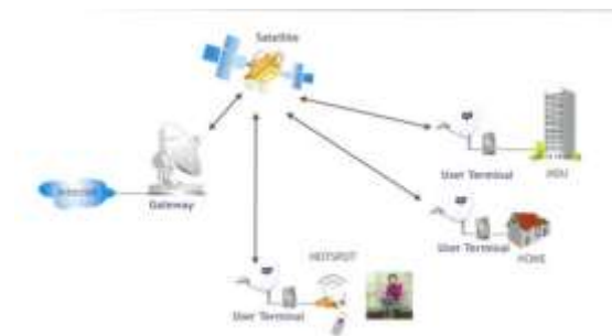
Figure 3.9 Architecture of the communication link viii. Future Set Up of VSAT At Customer Premises
