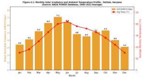
Fig. 2. Monthly solar irradiance (GHI) and ambient temperature profile (NASA POWER, 2000–2022).
