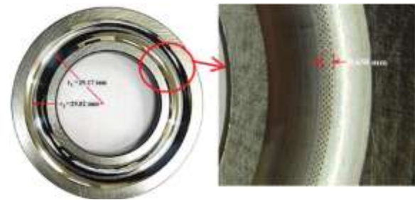
Fig.2. Textured outer race of test bearing, [46].
