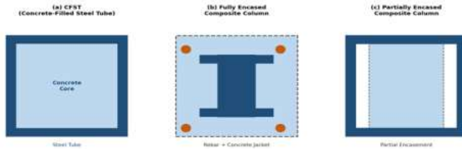
Fig. 2 – Cross-sectional configurations of steel–concrete composite columns: (a) CFST – Concrete-Filled Steel Tube; (b) Fully Encased; (c) Partially Encased [4].
