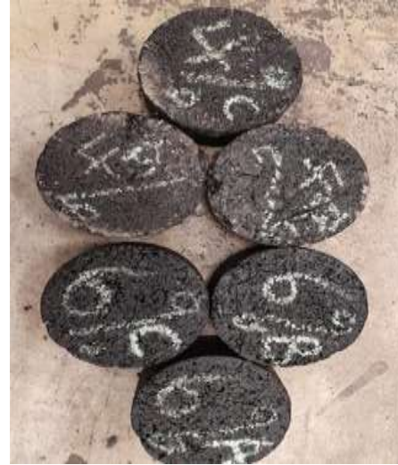
Figure 3: Pictorial presentation of PAM with 4% and 6% graphite content
