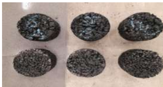
Figure 2: Pictorial presentation Porous Asphalt mixture pucks
