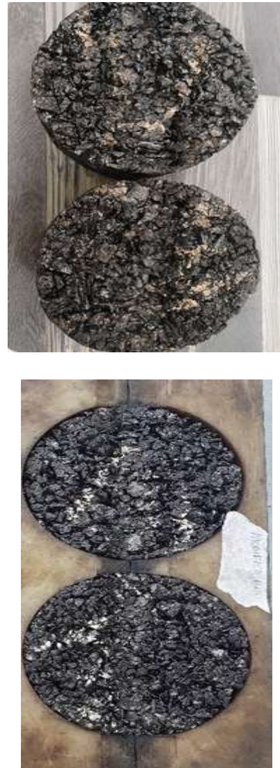
Figure 4: Pictorial presentation of rut of specimens of PAM
