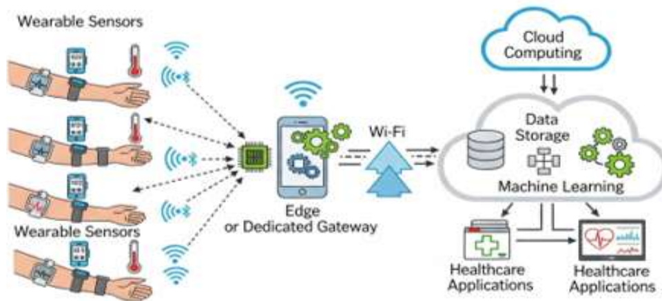
Figure 1. General architecture of a wearable IoT system for chronic disease monitoring
