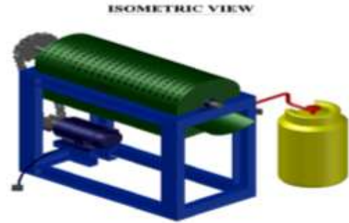
GAS POWERED GARRI FRYING MACHINE
