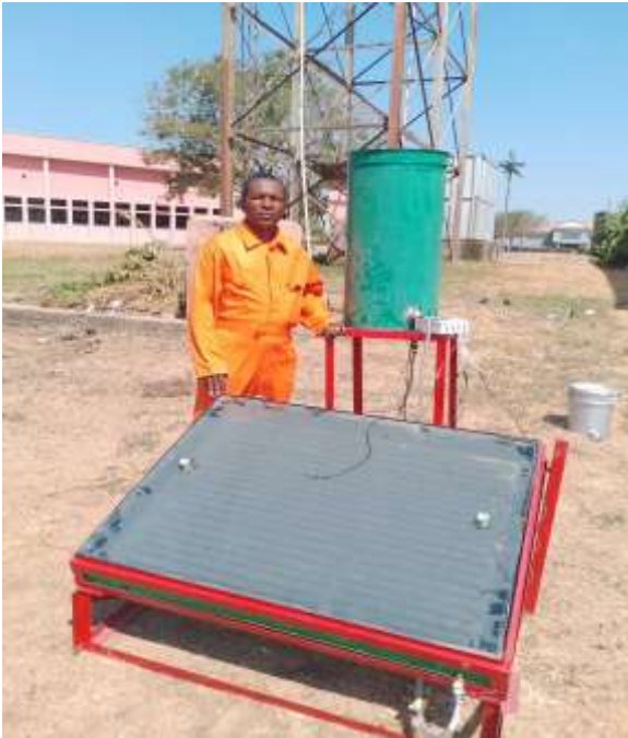
Figure 2 shows the photograph of the experimental flat-plate solar water heating system showing collector, storage tank, and instrumentation setup at Nigerian Defence Academy workshop.
