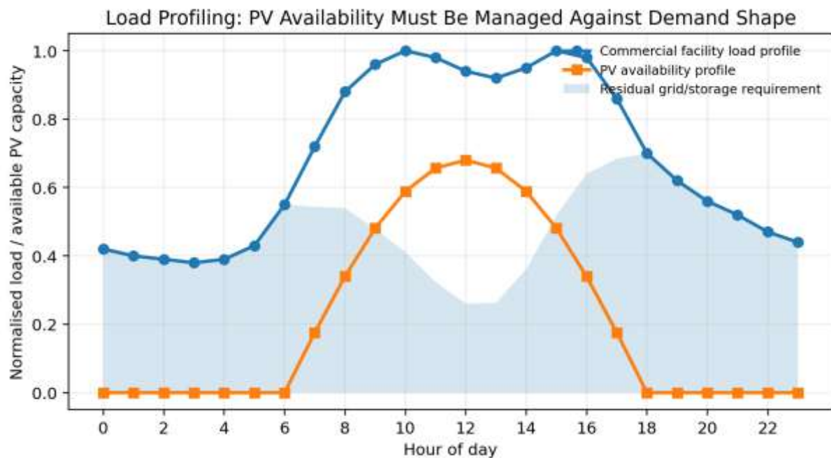
Figure 2. Conceptual load-profile and PV-availability matching for a commercial facility. Source: author model based on typical daytime facility load behaviour.
