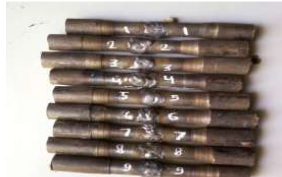
Fig. 2. ST-37 steel workpiece after bead-on-plate weld deposition, prior to sectioning for tensile testing.
