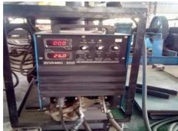
Fig. 1. Semi-automatic MIG welding machine used in the experimental programme.
