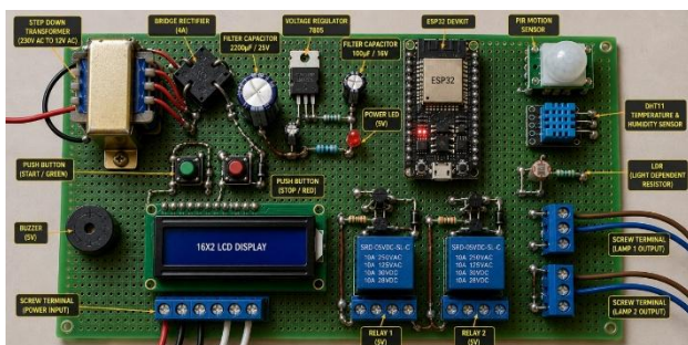
Figure 3. Completed PCB with ESP32, Power stage, Sensing Interfaces, Display, Buzzer, and Dual relays.
