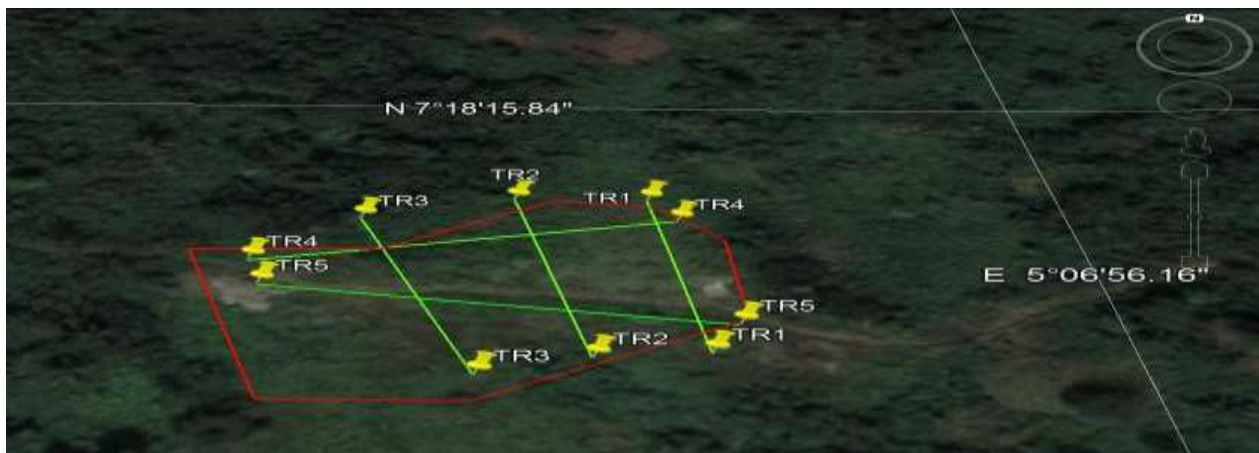
Figure 4: Layout of dipole-dipole traverses across the site
