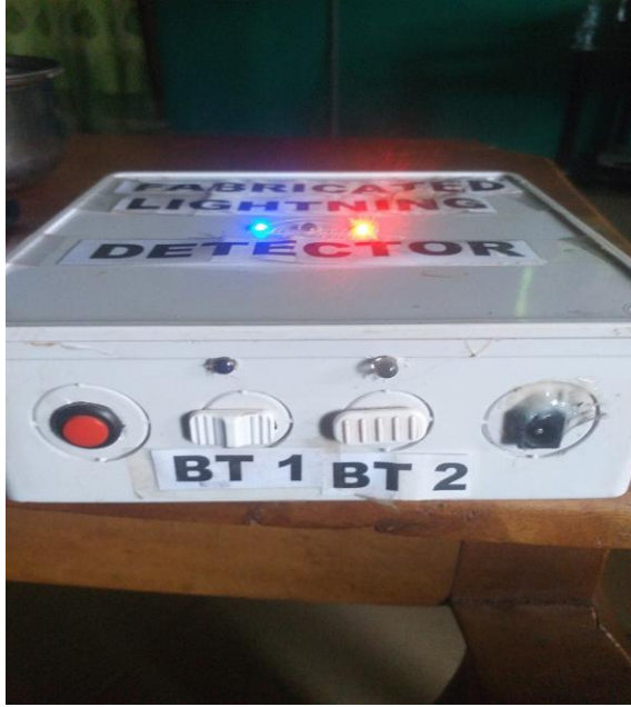
Figure 5: Fabricated Lighting Detector
