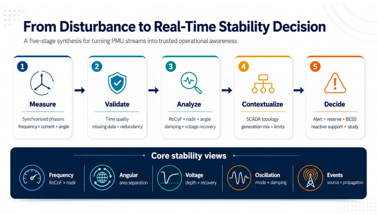
Figure 2. Five-stage PMU analytics pathway from disturbance measurement to an operator decision, with core stability views for frequency, angle, voltage, oscillations, and event propagation.
