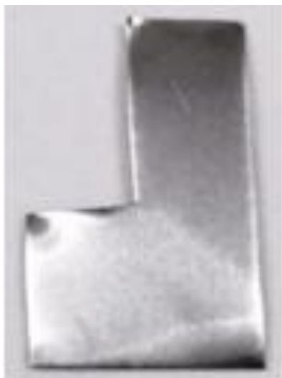
Figure 1. Ti foil cut into desired dimensions of 1×1 cm (1 cm extra was used as electrode holder)
