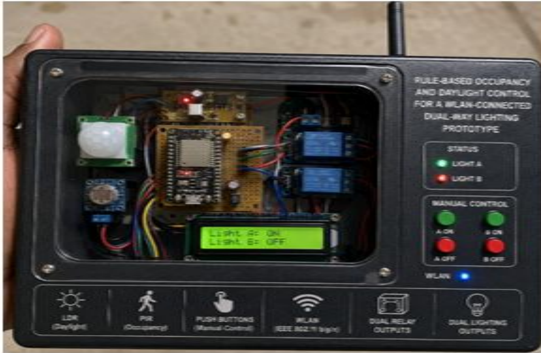
Figure 2. Enclosed prototype with two bracket lights, sensing modules, display, status indicators, and local controls.
