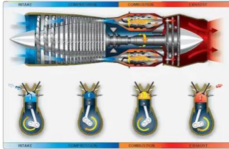
Figure 2.2: Gas Turbine operational stages - intake, compression, combustion, and exhaust (Aeronautics guide 2023)
