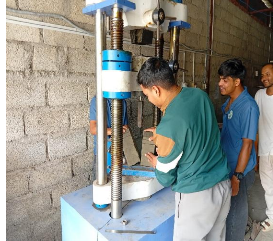
Fig: 3 Flexural Strength Test of Concrete Beam
