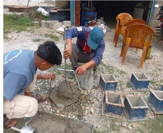
Fig 1: Slump Test of Concrete
