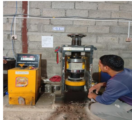
Fig 2: Compressive Strength test of Concrete Cube
