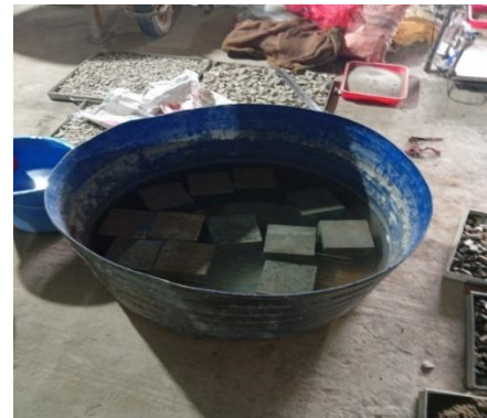
Fig 4: Water absorption test of Concrete Cube
