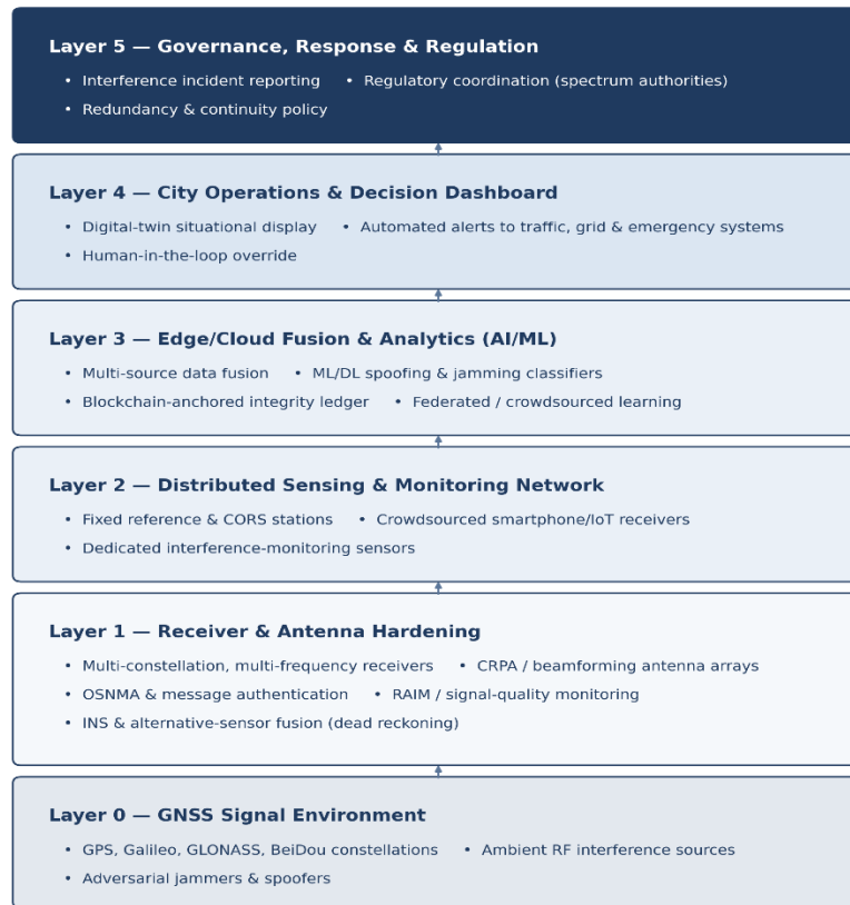
Figure 3. Proposed layered secure GNSS detection and mitigation architecture for smart cities.
