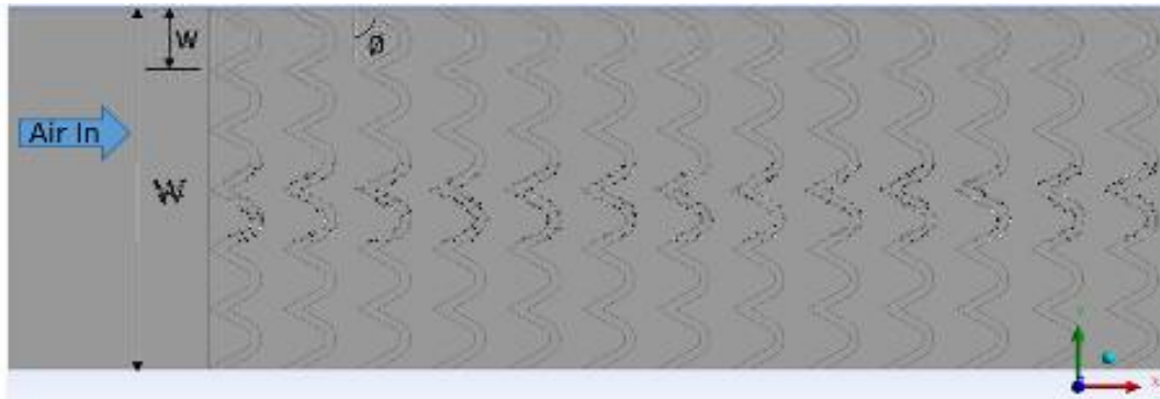
Fig. 2. Multiple V+arc roughness geometry.
