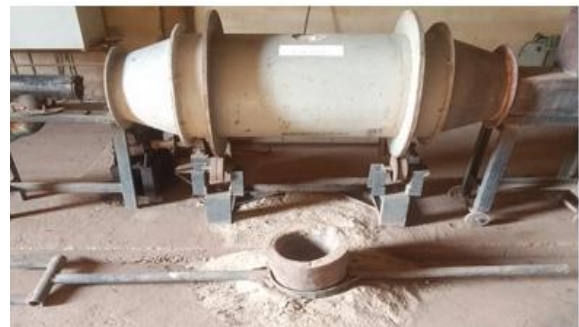
Rotary Furnace for melting metals
