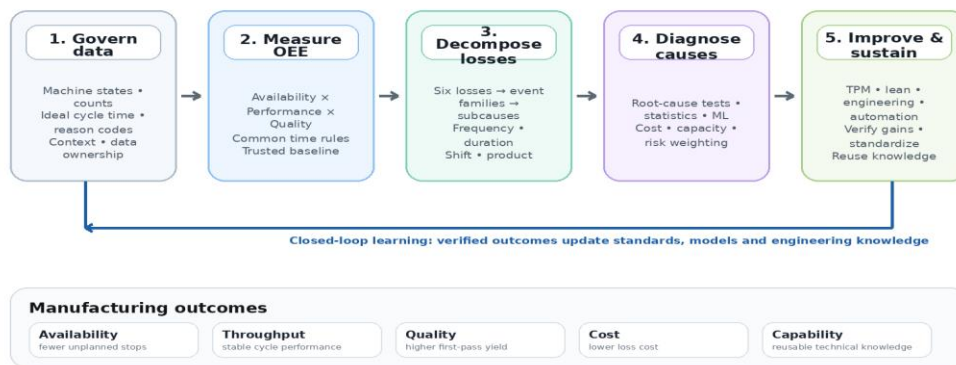
Figure 1. Integrated OEE and deep-loss machine performance management architecture.
