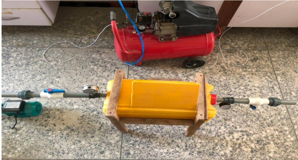
Figure 3.2: Core flooding system prototype Source: Researcher (2026)
