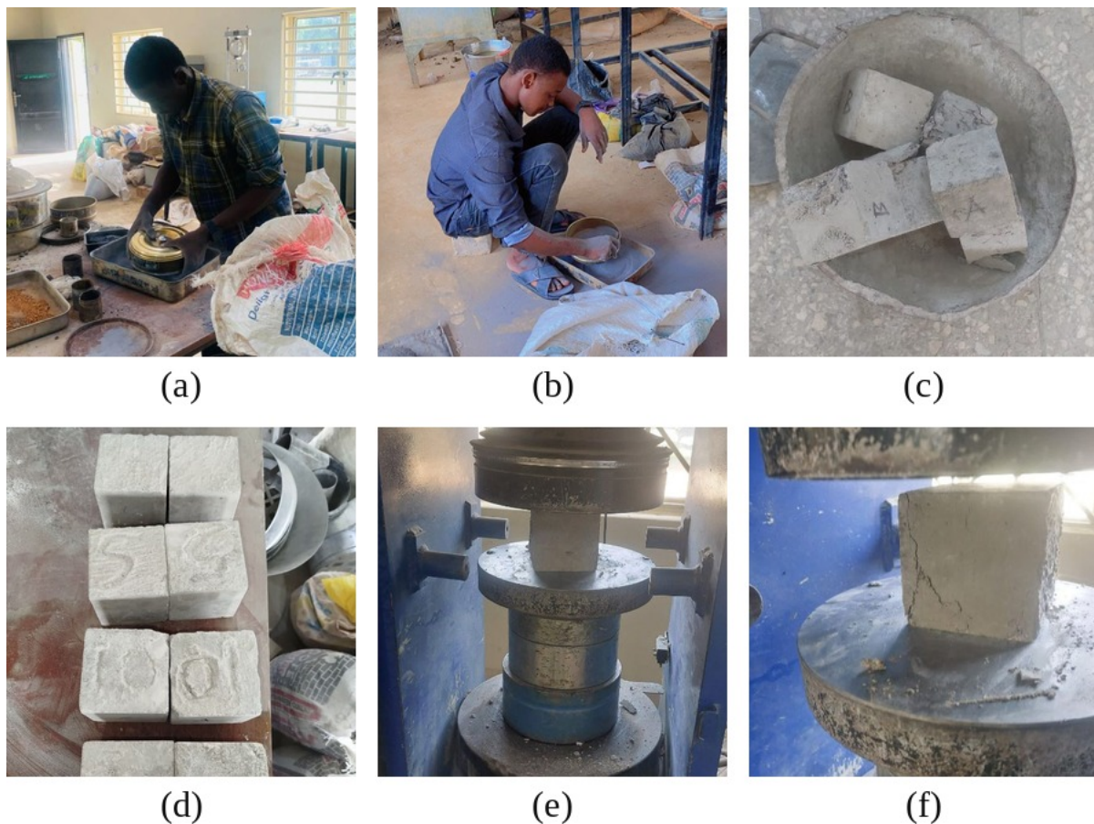
Figure 1. Experimental programme: (a) mechanical sieving; (b) manual sieving; (c) cubes after demoulding; (d) marked cubes ready for testing; (e) cube under load in the compression machine; (f) cube after the crushing test.
