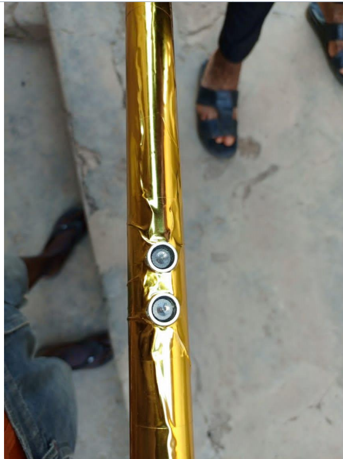
Figure 5. Placement of the ultrasonic sensor.
