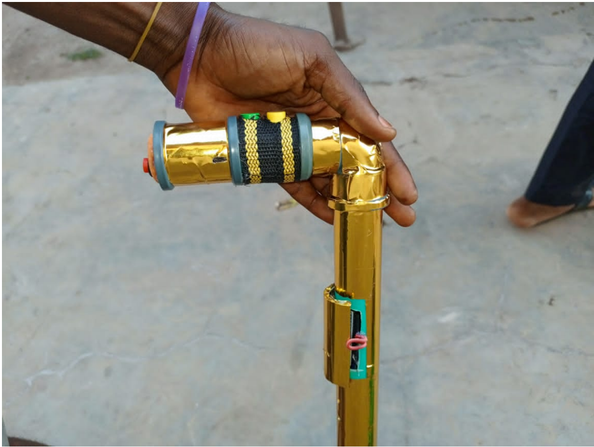
Figure 2. Smart blind stick assembly.
